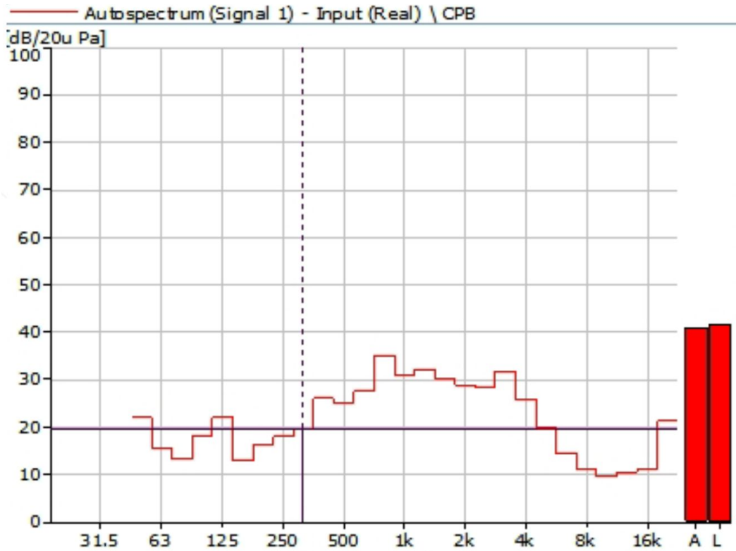
Figure 3 Noise Spectrum of Stage Luminaires (The Auto mode, Static, No 1)
